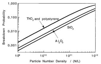
Fig. 3. Calculated breakdown probabilities as a function of the particle number density for different materials, normalized to a particle diameter of 30 nm.
