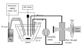
Fig. 2. Experimental setup of the coulometric pH titration cell.
