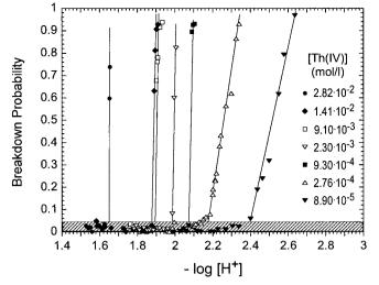
**Fig. 4.** Breakdown probabilities after background subtraction during the coulometric pH titration of  $2.8 \times 10^{-2} - 8.9 \times 10^{-5}$  M Th in 0.5 M HCl/NaCl at 25 °C.
