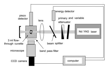
Fig. 1. Experimental setup of LIBD.
